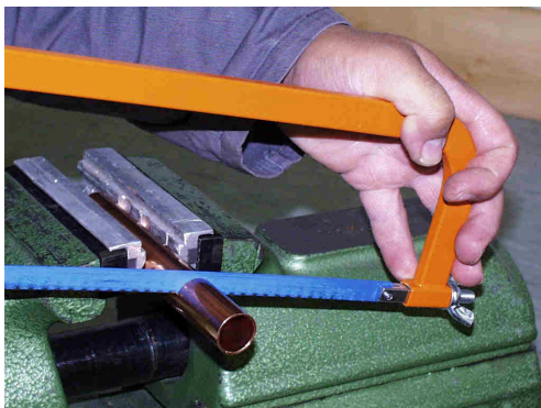
1. Rectangularly saw off the pipes
